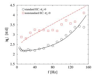
FIG. 11: (Color online) Modulus of the critical wave vector  $q_c$  as a function of frequency f for the compound 8/7 for positive as well as for negative  $\sigma_a$ . Experimental data (symbols) and theoretical results (lines).
