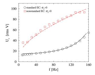
FIG. 10: (Color online) Experimental data (symbols) and theoretical results (lines) for the critical voltage  $U_c$  as a function of frequency f for the compound 8/7 for positive as well as for negative  $\sigma_a$ .
