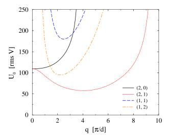
FIG. 9: (Color online) Neutral curves  $U_0(q)$  for the wave vector  $\mathbf{q} = (q, p)$  as a function of q at a fixed value of p for different magnitudes of the flexo coefficients  $(\xi_-, \xi_+)$  at  $\omega \tau_q = 0.5$ .
