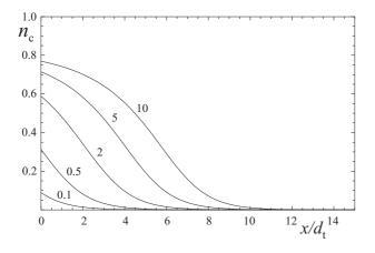
FIG. 7: The decay in *cis* number fraction  $n_{\rm c}(x)$  with reduced depth for various reduced incident intensities  $\alpha$  with  $\alpha/\beta = 5$ .
