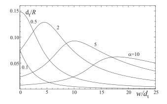
FIG. 8: Curvature reduced by  $1/d_t$  against reduced cantilever thickness  $w/d_t$  for various incident reduced light intensities  $\alpha$ (with  $\beta = 0$ ). For high intensities, bleached surface layers let light penetrate more deeply and hence a significant fraction of the cantilever has its natural length contracted. Bend occurs even for cantilevers much thicker than the linear penetration depth  $d_t$ .
