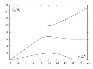
FIG. 10: Neutral surfaces for fixed incident light intensity  $\alpha = 5$  as cantilever thickness w changes. At the w maximising curvature, a third neutral surface appears from the rear face; at greater w a neutral surface is lost at the front face.
