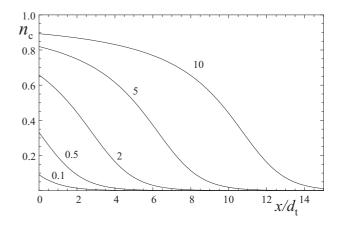
FIG. 5: The decay in *cis* number fraction  $n_{\rm c}(x)$  with reduced depth for various reduced incident intensities  $\alpha$ , with  $\alpha/\beta = 50$ .
