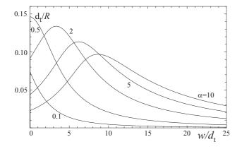
FIG. 9: Curvature reduced by  $1/d_t$  against reduced cantilever thickness  $w/d_t$  for various incident reduced light intensities  $\alpha$  (with  $\alpha/\beta = 5$ ). Maxima in curvature occur at smaller thicknesses than in the  $\beta = 0$  case where back reaction is purely thermal.
