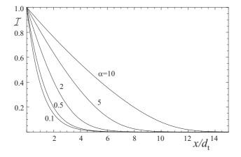
FIG. 4: The decay in reduced light intensity with reduced depth for various reduced incident intensities  $\alpha$ , with a weakly stimulated back reaction such that  $\alpha/\beta = 50$ . The plots are similar to those shown in figure 2.
