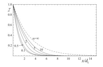
FIG. 6: The decay in reduced light intensity with reduced depth for various reduced incident intensities  $\alpha$  with  $\alpha/\beta = 5$ .
