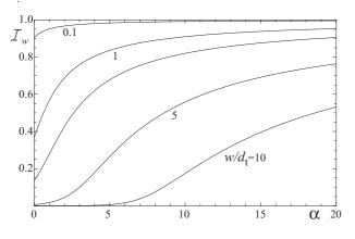
FIG. 11: Scaled intensity at the back surface  $\mathcal{I}_w$  as a function of the incident intensity  $\alpha$  with  $\beta = 0$  for various cantilever thicknesses  $w/d_t$ .
