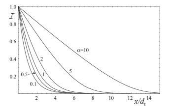
FIG. 2: The decay in reduced light intensity with reduced depth for various reduced incident intensities  $\alpha = I_0/I_c$ . Photo-induced back-reaction is minimal,  $\beta = 0$ .
