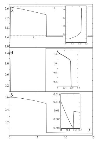
FIG. 13: Upper: Elongation  $\lambda$  for a cholesteric elastomer with  $\tilde{\mu} = 1/50$  illuminated by light of reduced intensity  $\tilde{I}$ . Middle: Director angle  $\theta$ . Lower: Order parameter S. Insets show the rapid variation and jumps at low intensities.
