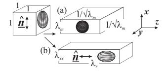
FIG. 1: An initially unit, cubical nematic elastomer (a) contracts on loss of order. The prolate spheroid characterizing the distribution of chains becomes spherical; (b) contracts along the original director, and elongates along the new, upon rotation by  $90^{\circ}$  of the director and thus of shape distribution.
