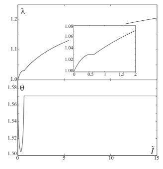
FIG. 12: Upper: The elongation along the helical axis for a cholesteric elastomer of  $\tilde{\mu} = 1/10$  illuminated with unpolarized light of intensity  $\tilde{I}$ . Lower: The associated rotation of the director away from the yz plane.
