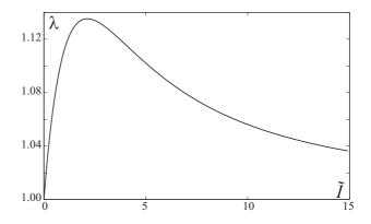
FIG. 9: The deformation  $\lambda$  along the beam propagation direction **k** as a function of the reduced intensity  $\tilde{I}$  of unpolarized light on an elastomer with  $\tilde{\mu} = 1/10$ .
