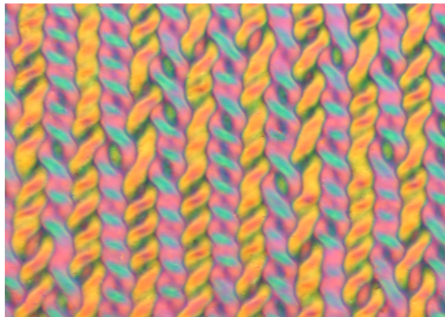
Figure 12: The “knitting” instability. It is produced by abruptly raising the voltage from one of the prewavy states.
