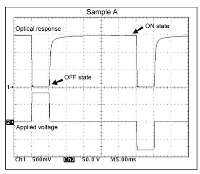
Figure 2: Oscilloscope snapshot of the applied field (channel 2) and the diffracted beam optical response (channel 1).
