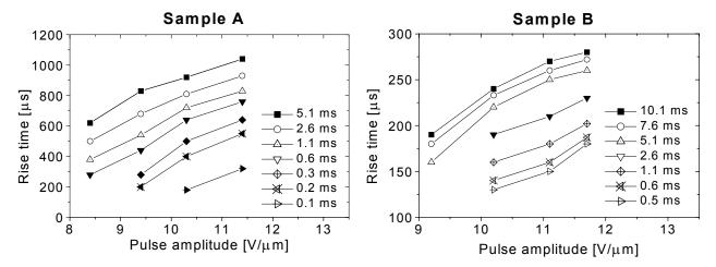
Figure 5: Same experimental points as in Figure 4; here rise time is reported versus pulse amplitude for different pulse durations.
