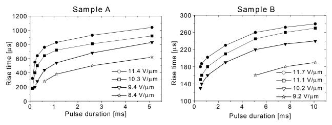
Figure 4: Rise time dependence on the pulse duration for different pulse amplitudes.
