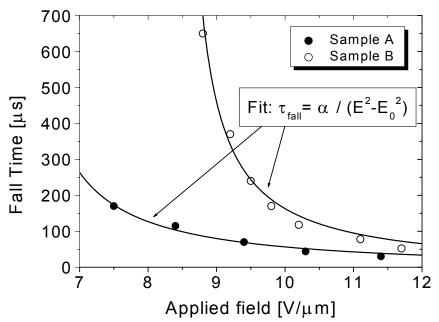
Figure 3: Fall time dependence on the applied field, experimental points and fit.
