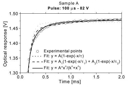
Figure 6: Diffracted beam optical signal (circles) during the off-on transition; lines show different fitting curves.
