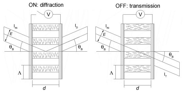
Figure 1: POLICRYPS operating model.
