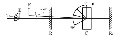
Fig.1: Scheme of experiment on the lasing threshold control in doped NLC. The orientation of E vector of pumping is vertical. The orientation of the NLC director n varies from vertical to horizontal by 84° angle with respect to polarization of pumping. The vector E of the lasing radiation changes synchronously with the orientation of NLC director. Reflectance of mirrors of resonator; R<sub>1</sub>=60%, R<sub>2</sub> = 100%.
