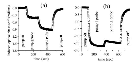
Figure 3: Change of the optical phase shift at pump intensity (a) 172  $mW/cm^2$  and (b) 656  $mW/cm^2$ .
