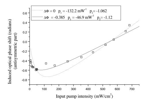
Figure 5: Difference in the optical phase shift as a function of input intensity. Open square: measured data. Dashed line: best fit with assuming  $\Delta \Phi_0 = 0$ . Continuous line: best fit, considering  $\Delta \Phi_0$  as a parameter.
