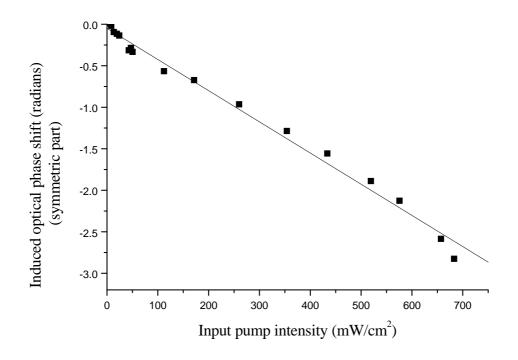
Figure 4: Average optical phase shift as a function of the input intensity.
