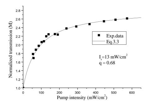
Figure 2: Nonlinear probe transmission normalized to the linear transmission. Squares: measured data. Continuous line: fit according to Eq. (3). The intensity values here and in subsequent figures refer to the peak intensity of the pump beam, calculated as  $I = P/\pi r^2$ , where *P* is the pump power and *r* is the pump 1/e radius (1mm).
