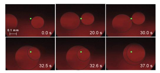
Figure 5: Manipulation of islands on an 8CB film. First, the laser, indicated by the green dot, is used to trap the island on the right. A second island is then brought close to the trapped island by translating the entire film (to the right). When the two islands are maneuvered close enough together, they coalesce. The edges of the islands have been highlighted here for clarity.
