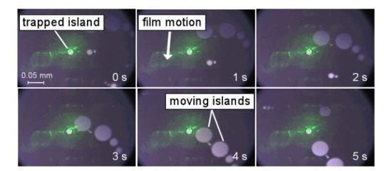
Figure 4: Optically trapped island (circled) in a moving film of MX8068. The laser beam is seen as a bright green dot near the edge of the trapped island. The elapsed time between frames is 1 second.
