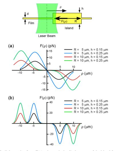
Figure 6: (a) Radial trapping force  $F(\rho)$ , where  $\rho$  is the displacement of the island from the center of the beam, computed for various island radii R and thicknesses h, assuming P = 250 mW,  $\kappa = 2.4$ , n = 1,  $\lambda_0 = 514.5$  nm,  $w_0 = 5$  µm, and a film thickness d = 0.05 µm. (b) Trapping force with narrower beam waist ( $w_0 = 2$  µm).
