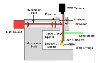
Figure 2: Experimental setup for observation and optical trapping of islands on smectic films and bubbles. Bubbles are inflated from LC material covering the tip of a hypodermic needle by slowly injecting air through a micro syringe.
