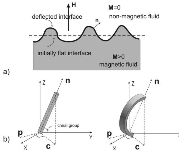
**Figure 1. (a) Instability of the interface between a magnetic fluid confined together with an immiscible non-magnetic fluid, the external magnetic field  $H$  is perpendicular to the undisturbed interface; (b) definition of the directors in the smectic- $C^*$  (left) and in the smectic-CP phase (right);  $c$ -director is the direction of the molecular tilt, the  $p$ -director shows the direction of the local spontaneous polarization.**
