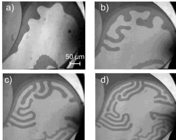
**Figure 3. Onset of the instability and development of a labyrinthine pattern (a)-(d) in absence of external electric fields at a constant heating rate 1 K/min, the time between subsequent images is 40 s**
