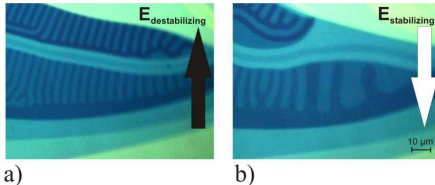
**Figure 5.** The electric field perpendicular to the boundary favors finger growth (a); the electric field of the opposite polarity makes the fingers shrink and disappear (b) (smectic-X phase, 146°C)
