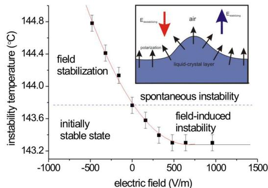
**Figure 6. (a) Stabilizing and destabilizing effects of the external electric field on the onset temperature (points denote the onset of fingering, the curve guides the eye); (b) fingering in a homogeneously polarized film. The p-director (direction of the polarization) is perpendicular to the boundary. Application of external electric field antiparallel to the p-director favors its splay.**
