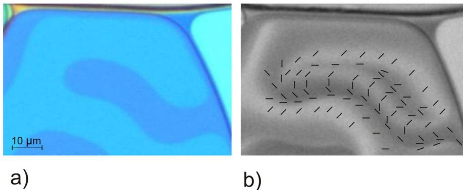
**Figure 4. The c-director field within the finger between slightly decrossed polarizers (a), and the same image without the polarizers (b) (smectic-X phase, 147°C). The p-director is at right angle to the c-director (i.e. perpendicular to the boundary)**
