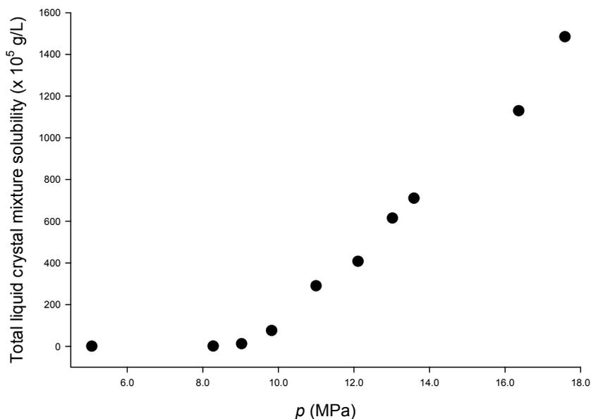
**Figure 6: Total liquid crystal mixture solubility as a function of pressure in supercritical CO<sub>2</sub> at 313.15K.**
