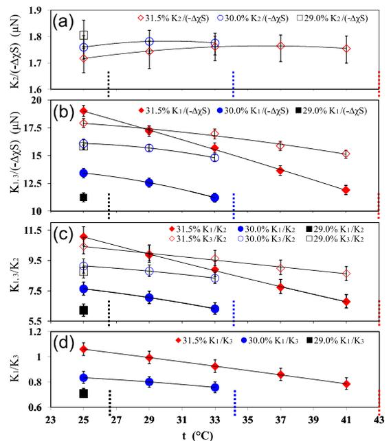
FIG. 3: (color online) Temperature and concentration dependences of (a)  $\frac{K_2}{-\Delta\chi S}$ , (b)  $\frac{K_{1,3}}{-\Delta\chi S}$  and (c)  $K_{1,3}/K_2$ . (d)  $K_1/K_3$
