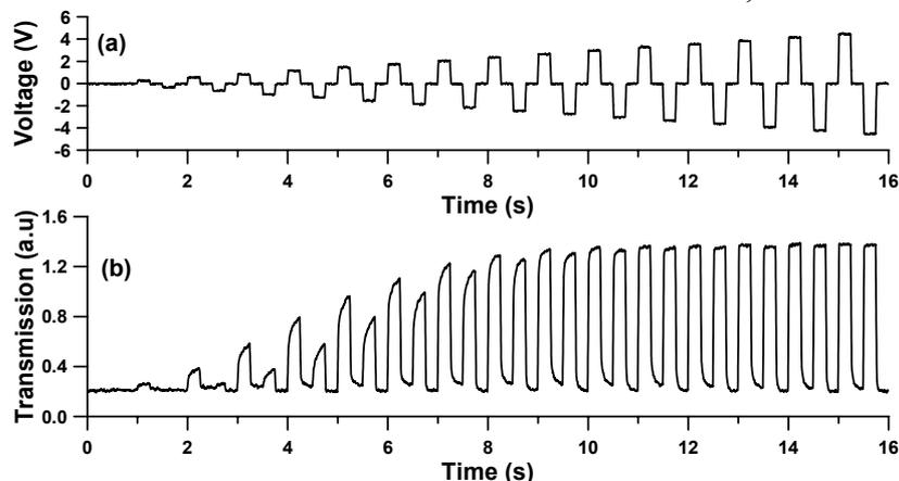
Figure 4: Driving waveform (a) and the grayscale obtained (b) in the time domain.
