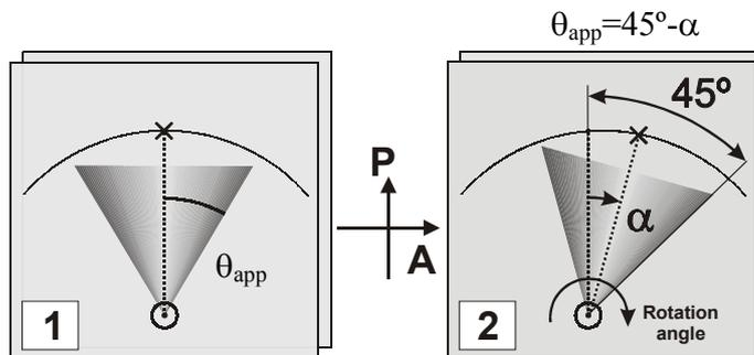
Figure 1: Measurement of the apparent tilt angle.
