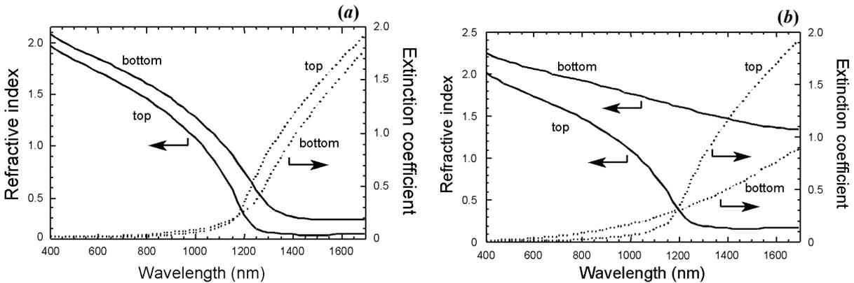
Figure 7a-b. ITO layer refractive index and extinction coefficient versus wavelength for fit 2 (a) and fit 3 (b).
