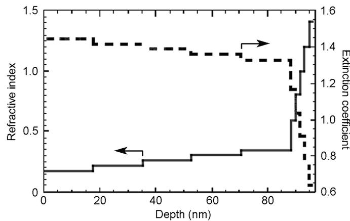
Figure 8. Optical constants profile for the ITO layer at  $\lambda=1500$  nm (fit 3). Depth=0 corresponds to air-ITO interface.
