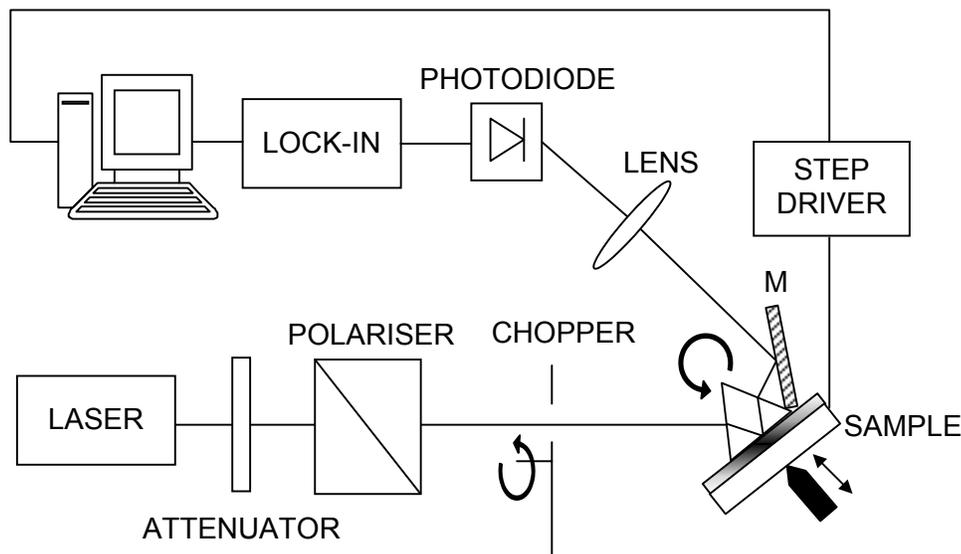
Figure 1. M-lines set-up.
