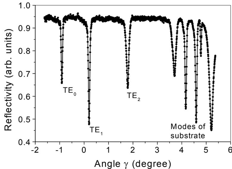
Figure 6. Angular spectrum of TE guided modes obtained by m-lines method for the TeraHertz sample ( $\lambda = 633 \text{ nm}$ )
