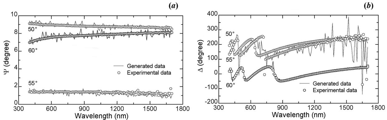
**Figure 2a-b.** Spectroscopic ellipsometric measurements for the 5CB liquid crystal sample:  $\Psi$  (a) and  $\Delta$  (b) experimental data and respective generated curves (fit 1) for 50°, 55° and 60° incidence angles.
