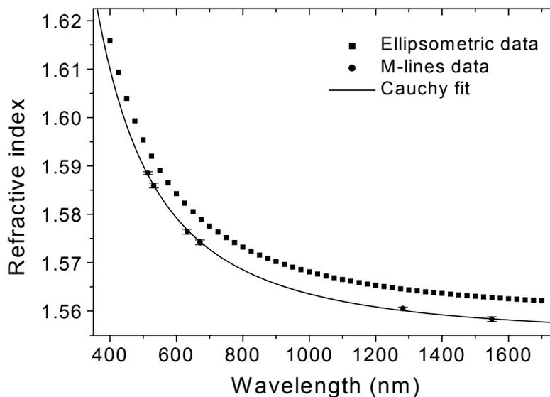
Figure 5. Results of ellipsometry and m-lines optical characterisation of CS-GMA polymer planar waveguide.
