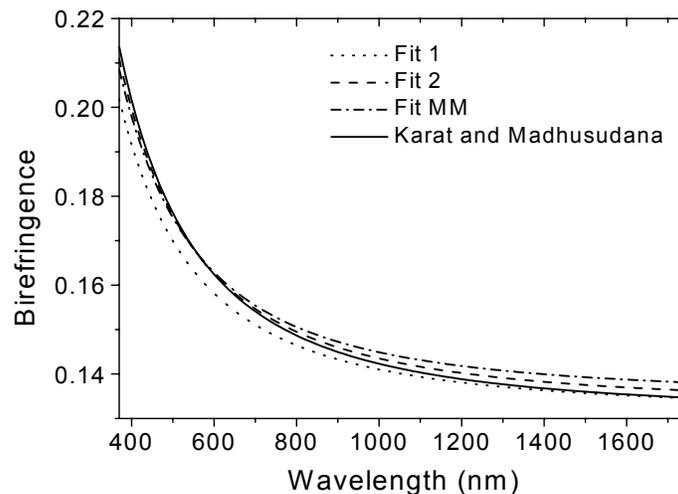
Figure 4. Birefringence dispersion for 5CB LC: the curves refer to three fitting procedures and one literature data set.
