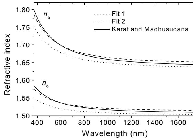
Figure 3. Ordinary and extraordinary refractive index dispersion for 5CB liquid crystal: the curves refer to two fitting procedures and one literature data set.
