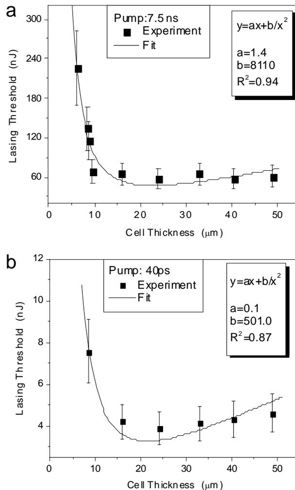
**Fig. 6** Lasing threshold as function of sample thickness. (a) nanosecond pump (b) picosecond pump
