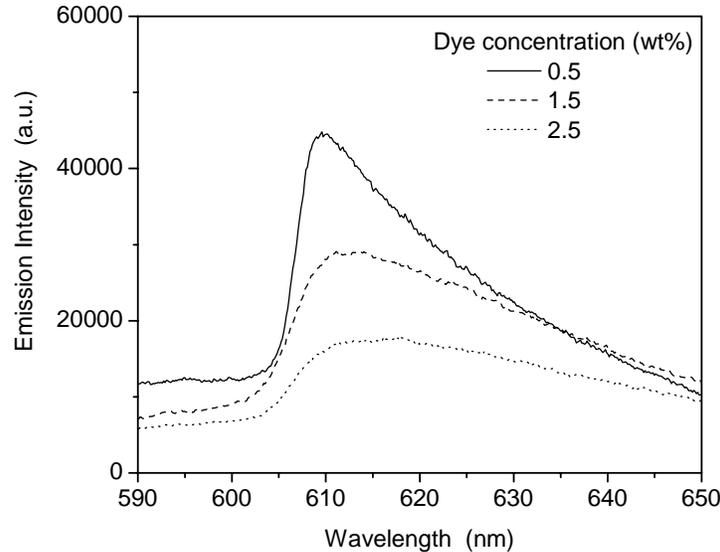
**Fig. 3** Fluorescence quenching: fluorescent emission for different dye concentrations. The pump pulsewidth is  $7.5\text{ns}$ .
