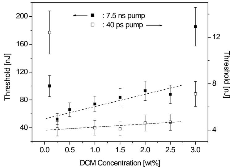
**Fig. 2** Dependence of lasing threshold on dye concentration with nanosecond and picosecond pump pulses. The dotted lines are linear fits in the concentration region of 0.25 wt% to 2.5 wt%.
