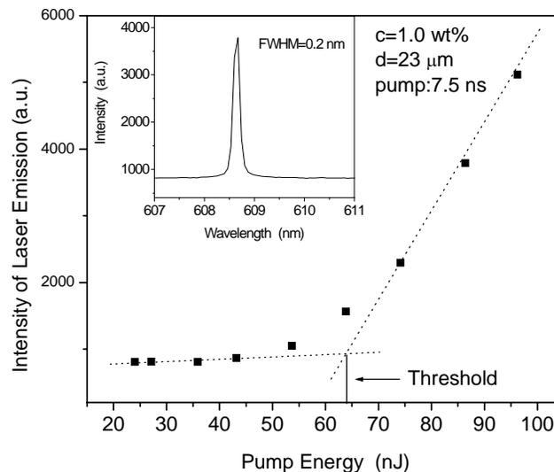
**Fig. 1** Intensity of CLC laser emission as function of pump energy.
