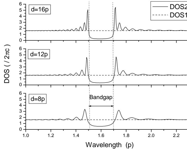
**Fig. 7** Calculated DOS for the two normal modes as a function of cell thickness. The dotted lines are the reflection band edges of a semi-infinite sample,  $n_o = 1.51$ ,  $n_e = 1.70$ .
